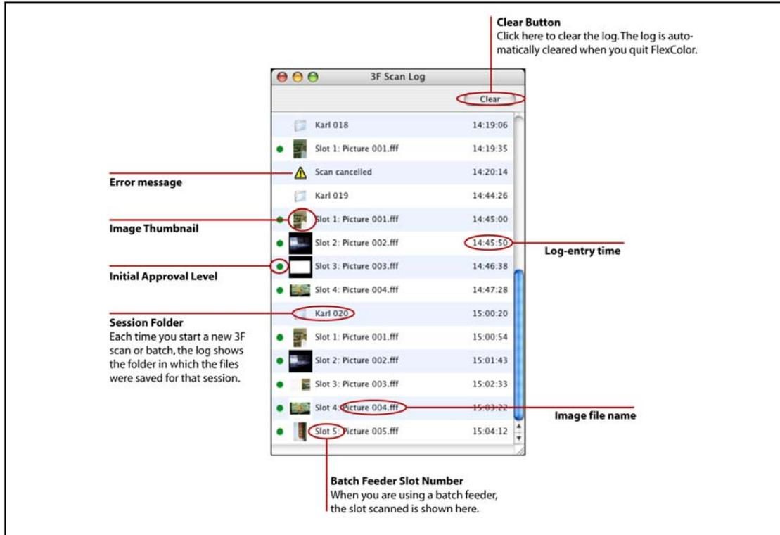
Figure 8: Features of the 3F Scan Log window.
